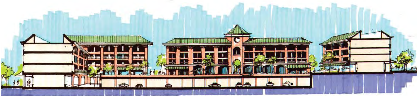
Figure 3.13: Cross-Section of Potential Redevelopment between Cooper and Centre Streets The change in grade between the new parallel connector street and the railroad station may allow for multi-story parking accessed on both levels.
