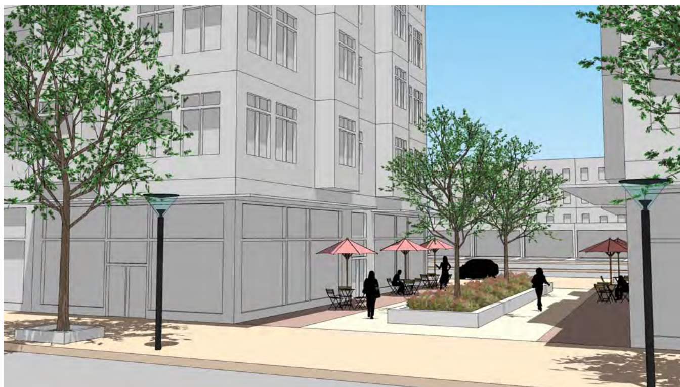
Figure 4.12: Mid-block cut-through provides pedestrian access to parking lots located to the rear of buildings
